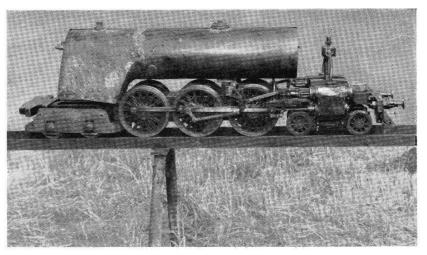
MR. CI.ARK'S model R class in embryo . . the forerunner of others. Most of the job will be done from V.R. blue-prints. It has been successfully tested on air, and the smoke box and pipe connexions are being completed before making a steam test.
