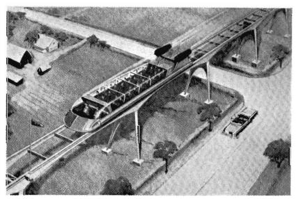
Levacars, guided by rails, supported and propelled by air, might be used, as shown in the artist's' conception above, for passenger transportation at speeds of 200 to 500 miles per hour.
