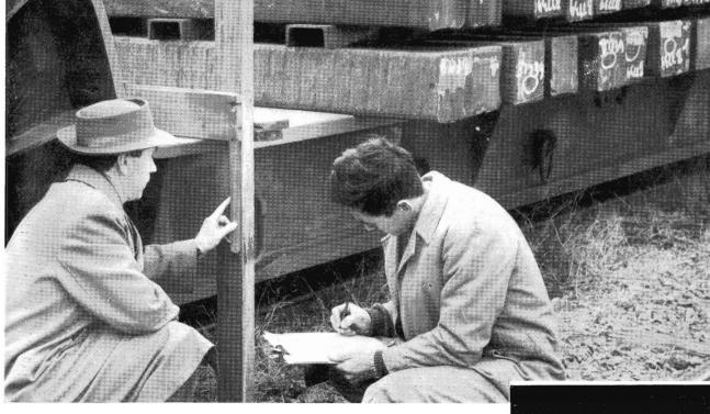
Rolling Stock Branch Engineers G. McMahon and N. Hill checking deflection, under load, of well wagon that is nearing completion at Newport Workshops. Designed to carry massive stators for the State Electricity Commission, as well as other special loads, the wagon will have a capacity of 150 tons and is the biggest of its type ever built by the Department.
