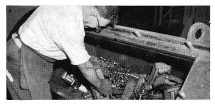
Removing brake blocks from drum of rumbler, after cleaning has been completed.
