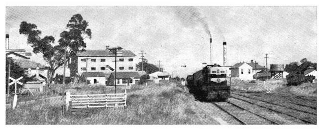
Factory buildings of the Railways two biggest customers at Maffra—(left) The Maffra Co-operative Milk Products Co. Limited and Nestle Co. (Australia) Limited—flank the arriving goods train hauled by the latest type T class diesel electric locomotive from Traralgon.
