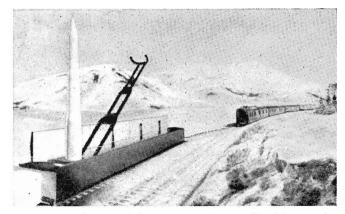
At the firing point, the missile wagon would be cut off and the rest of the train pulled clear.
