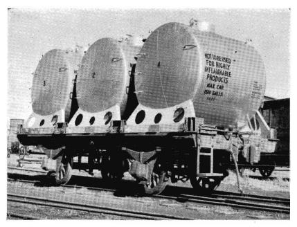
To meet this demand special concontainers fitted with internal steamheating coils have been provided. The containers have a capacity of 1,510 gallons (nearly six tons) of tallow and are carried on special KC wagons.
