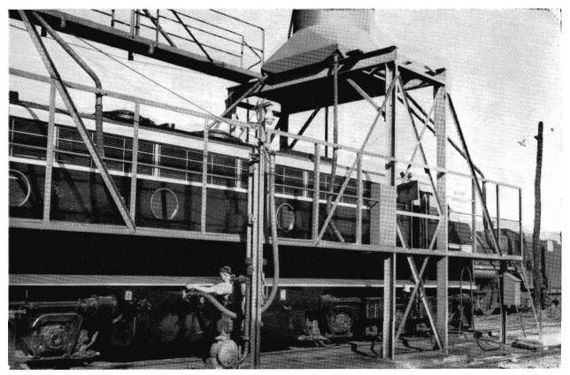
Diesel-electric locomotive re-fuelling at North Melbourne Diesel Workshops.
