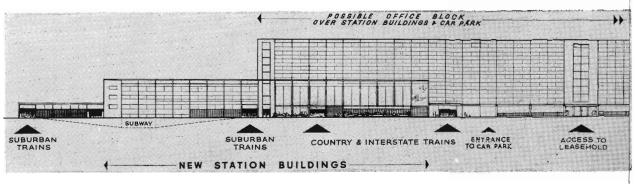
NEW interstate train terminal for Spencer Street, with possible extension of the building by erection of a multi-storey office block through leased "air-rights."
