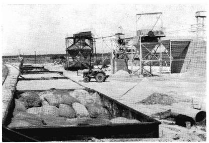
Trucks loaded with bulk and bagged shell grit, with the production plant in the background. The trucks are standing in the loop specially built to serve the industry.
