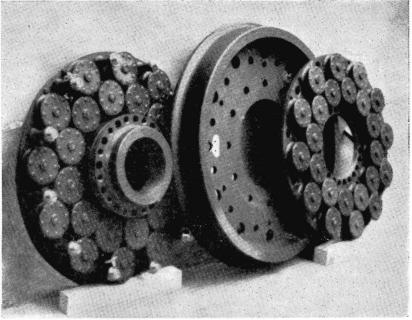
Metal discs and circular rubber blocks used in resilent wheels.
