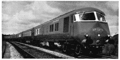
Eight-car diesel-electric Pullman train on trial run.
