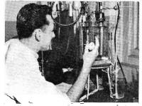
Every care is taken to ensure that the best value is obtained when stores are bought. Materials of various kinds—such as steel, oil, paints, canvas, etc.—are tested, before purchase, by staff under the Engineer of Tests at Newport Workshops Laboratory. Picture shows a chemist at the Laboratory ascertaining the viscosity of a sample of oil.
