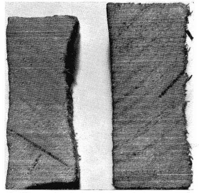
(Above) TIMBER specimens showing (left) an air-dried piece in which timber cells have partially collapsed, causing a distorted and wasteful cross-sectional shape. The other piece of timber has been through the steam chamber and has returned to its original shape and availability for complete machining. (Below) METER readings of moisture content (before treatment of the timber) being taken by Foreman F. Tongue.
