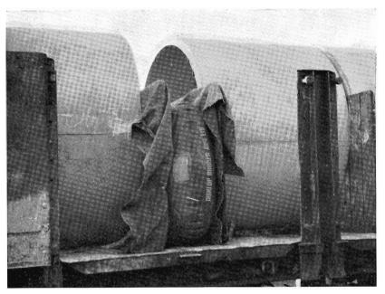
Pneumatic dunnage between concrete pipes.
